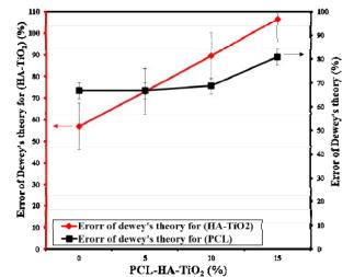
Fig. 8. The percentage error in Dewey's theory for nanoparticles (HA, TiO<sub>2</sub>) and polymer (PCL)
