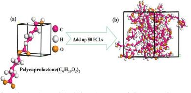
Fig. 5. (a) Polycaprolactone polymer with double chain PCL structure and (b) Composite polymer simulated in the materials studio software.
