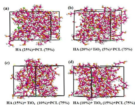
Fig. 6. MD simulation of bio-nanocomposite containing of (a) 0 wt%, (b) 5 wt %, (c) 10 wt%, and (d) 15 wt % of TiO<sub>2</sub> in the HA and PCL microstructure simulated in the MD software for orthopedic approaches.
