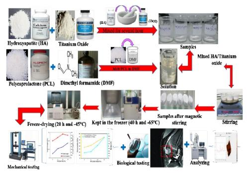
Fig. 1. Schematic of PCL bio-nanocomposite scaffolds made by the freeze-drying method with HA and TiO, nanoparticles.
