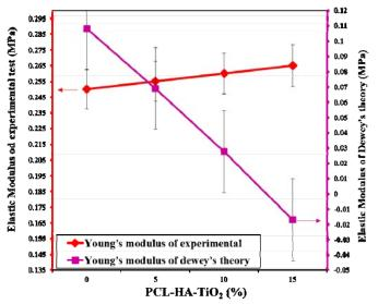
Fig. 7. Comparison of the Elastic modulus obtained in the experimental with Dewey's teaory.
