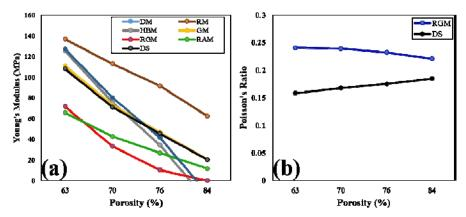
Fig. 9. Comparison between the experimental results and micromechanical modelling of elastic modulus of porous synthetic bone scaffold in this study by means of (a) DM, RM, HBM, GM and RAM, RGM and DS (b) the obtained Poisson's ratio of RGM and DS model.
